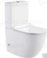
GD2204P-PT4 Washdown two-piece toilet Size: 620X380X825mm S-trap: 100/250mm Roughing-in P-trap: 180mm Roughing-in UF Seat cover
