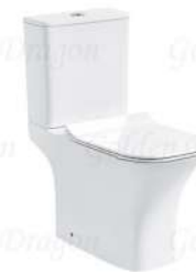
GD2205-PT5 Washdown two-piece toilet Size: 665X355X770mm S-trap: 250mm Roughing-in P-trap: 180mm Roughing-in
