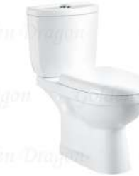
GD2020 Washdown two-piece toilet Size: 700X380X740mm S-trap: 250mm Roughing-in P-trap: 180mm Roughing-in
