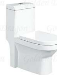
GD2135 Washdown one-piece toilet Size: 720X370X790mm S-trap: 250mm Roughing-in P-trap: 180mm Roughing-in
