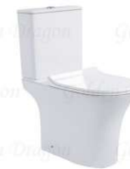
GD2206-PT6 Washdown two-piece toilet Size: 665X355X770mm S-trap: 250mm Roughing-in P-trap: 180mm Roughing-in
