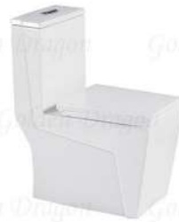
GD2226 Washdown one-piece toilet Size: 650X370X760mm S-trap: 250mm Roughing-in UF Seat cover
